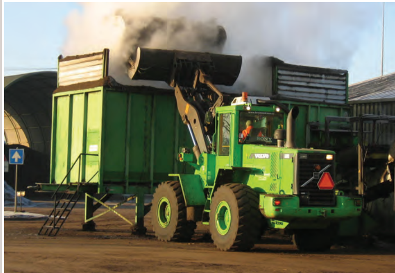
Support Structures Provides the required 3' minimum maintenance access under the bin. Concrete supports or pit mounting are also options.
